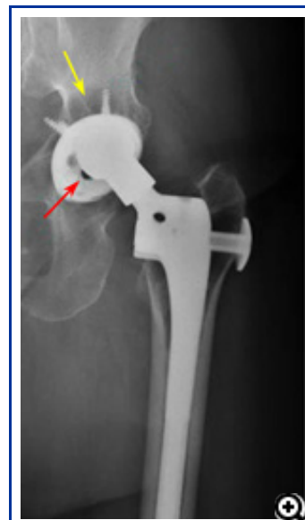
Wear of the plastic liner (red arrow) and osteolysis (yellow arrow) have caused the acetabular cup to loosen. The femoral head (ball) is no longer centered in the cup.
